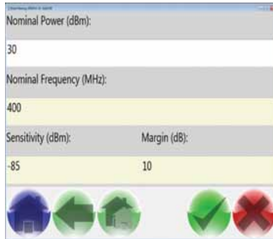
Figure 2: Radio parameters screen in PnC. The simple interface requires minimal input from the user.
